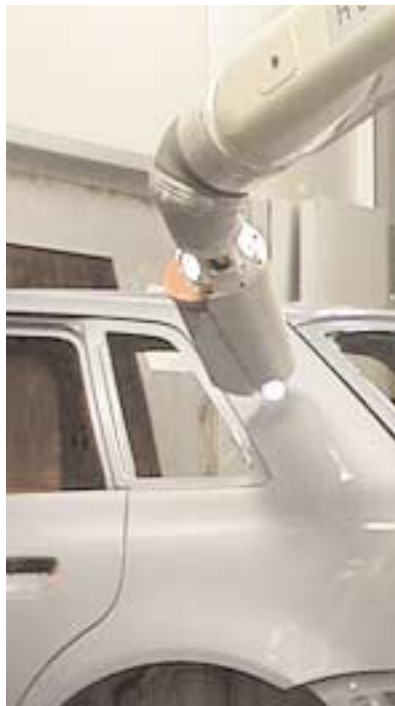
Figure 1: The robot moves the laser measuring system to any point on the body.
