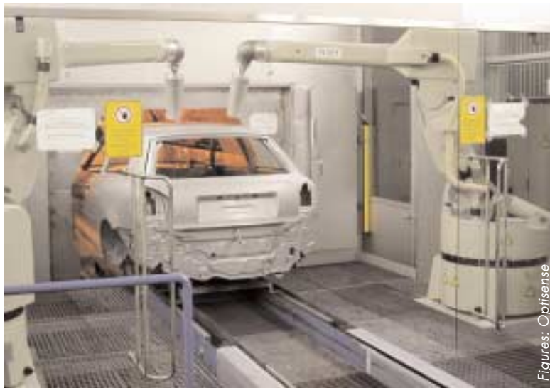
Figure 2: Synchronous scanning of the freshly coated body using two six-axis robots in tracking operation (throughput operation)
