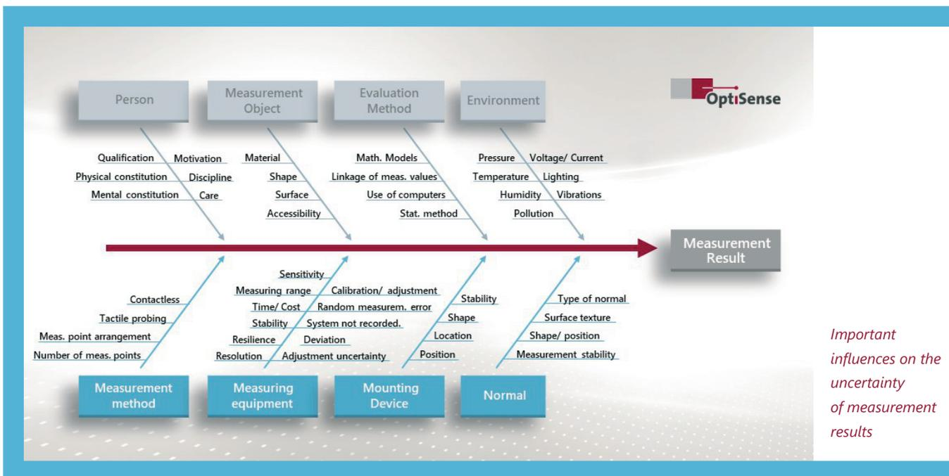
This can be used to estimate whether the coating thickness measuring system is even an option. The components influencing the measurement process are evaluated with standard uncertainties  $\mu$  and presented in an uncertainty budget, for the completeness of which the user is responsible. So the subject is complex.
